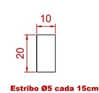
**VIGA CINTA (PLATIBANDA)**
